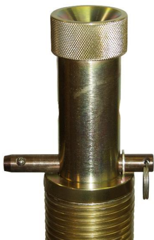
Washer In Ram Protection Ring
