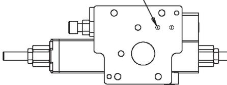
Figure 7. "P-1NN" and "P-LNN" Control Drain Port Location
