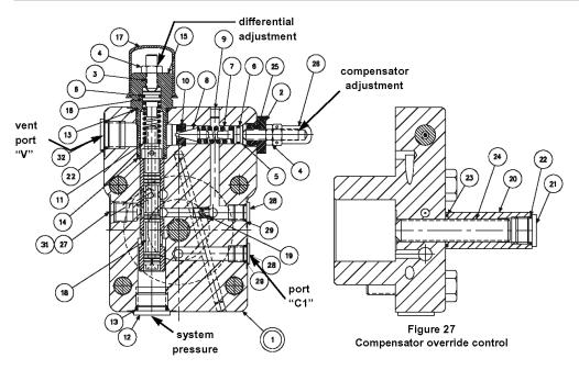
PARTS LIST FOR FIGURE 27 compensator override control P07 compensator override S22-16205 P110 comp. override S22-16206
