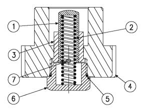
FIGURE 9 Buck-up cap assembly
