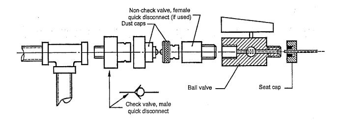
Figure 1 — Typical field type sampling device
