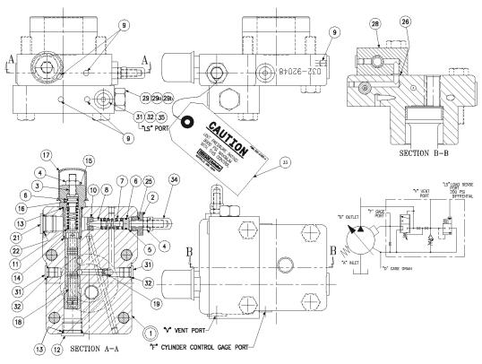
Ref. Figure 12 load sensing compensator control
