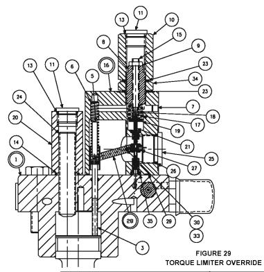
PARTS LIST FOR FIGURE 29 torque limiter override P07 code J, S22-16207 P07 code K, S22-16209 P110 code J, S22-16208 P110 code K, S22-16210
