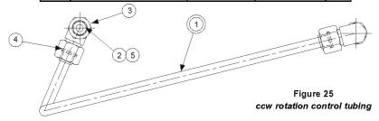
**PARTS LIST FOR FIGURE 25** ccw rotation control tubing S22-16036 (P07) S22-16038 (P110)
