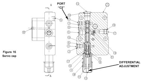
ADJUST FOR ZERO FLOW AT 175 MA ELECTRICAL COMMAND
