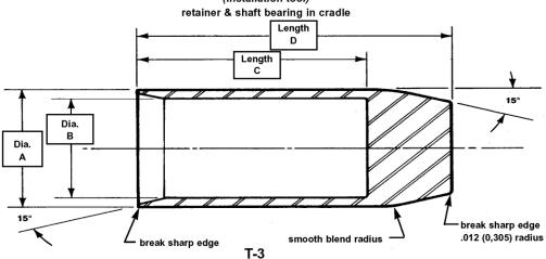
(installation tool) shaft seal over shaft
