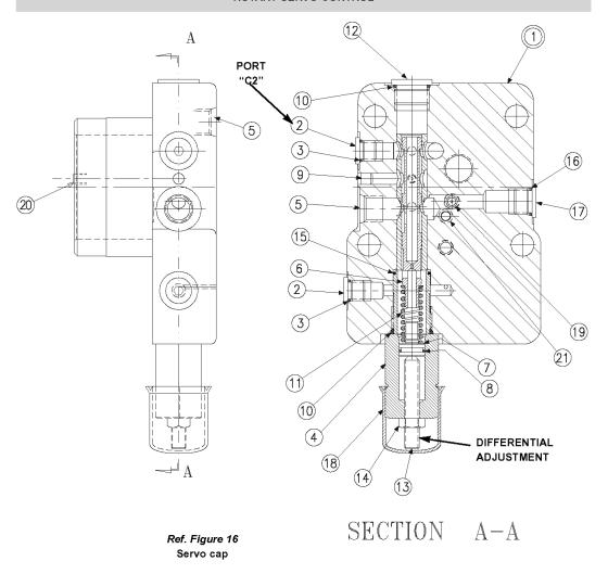
PARTS LIST FOR FIGURE 16 P07 servo cap S22-16063 P110 servo cap S22-16064
