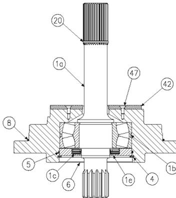
28. Install retaining ring (20) on shaft.
