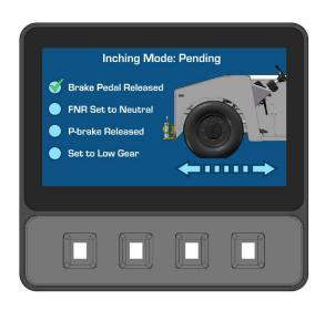
To inch, press and hold the inching switch in the desired direction. The tractor will roll in the requested direction for as long as the switch is pressed, up to a maximum value. If additional inching travel is required, release and then re-press the switch.
